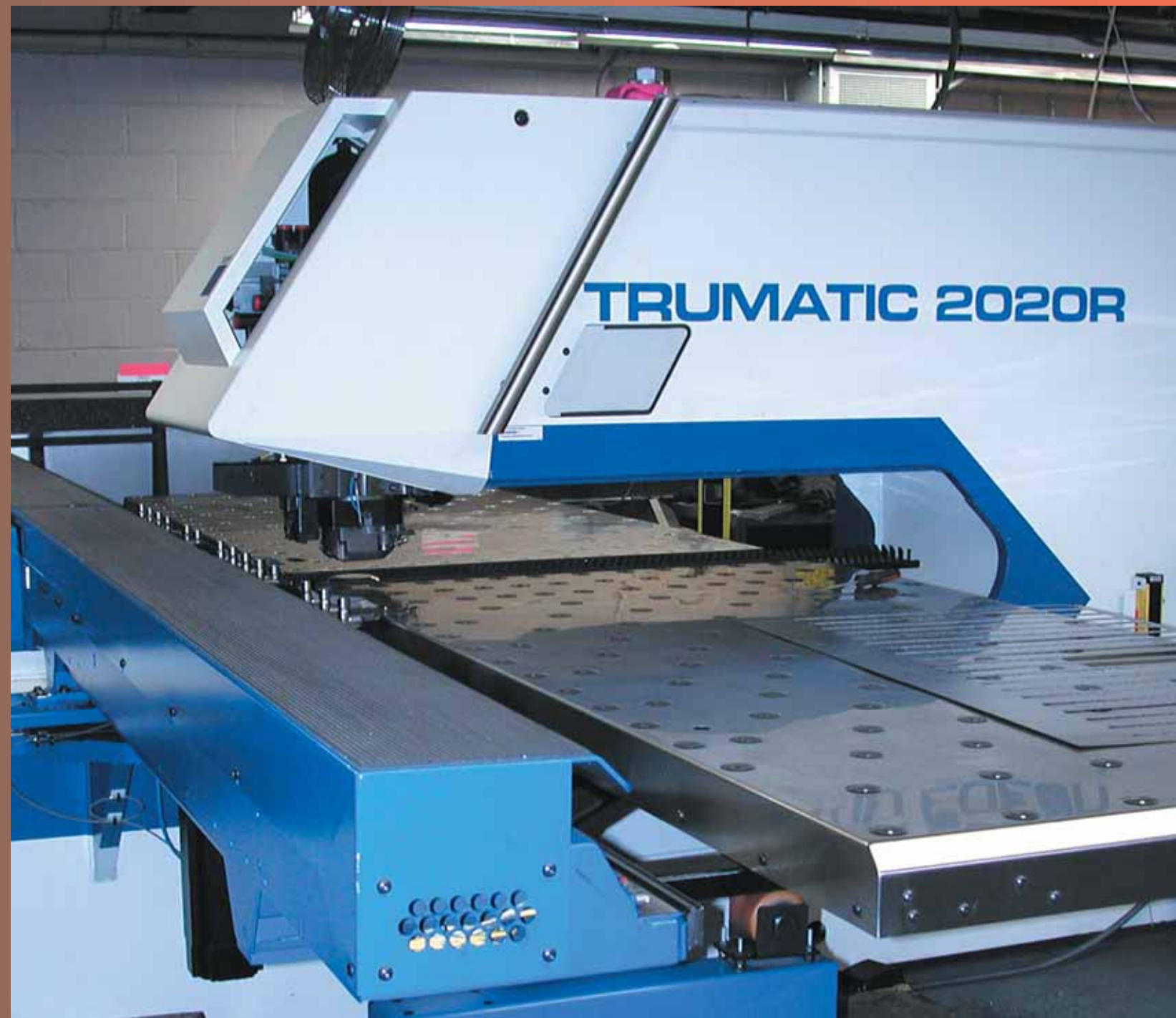
TRUMATIC 2020R Press—a high-precision coordinate-holing sheet-processing center with numerical program control.
