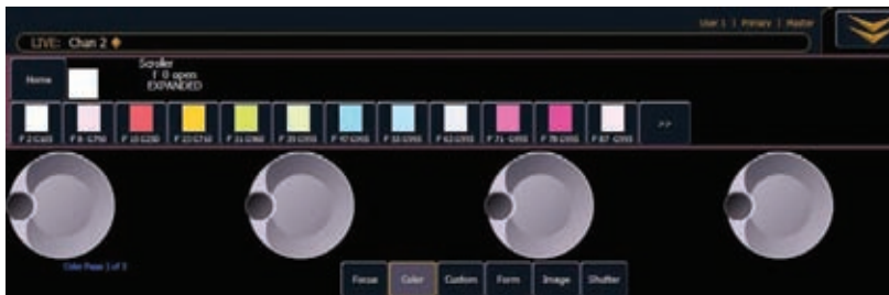
Figure 5: EOS Console showing gel colors read via ACN-RDM
