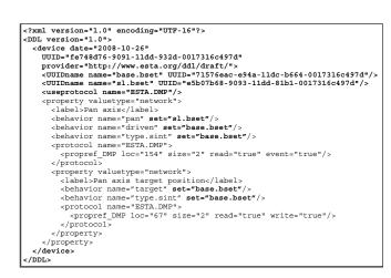
This is now a complete device description and validates against a DDL schema (see sidebar "Validating DDL" on page 25). However, it only describes one axis of the light and does not convey much detail.
